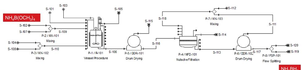
Figure 3. Process 2 - Recovery process from ammonium methoxyborate to pristine ammonia borane.
