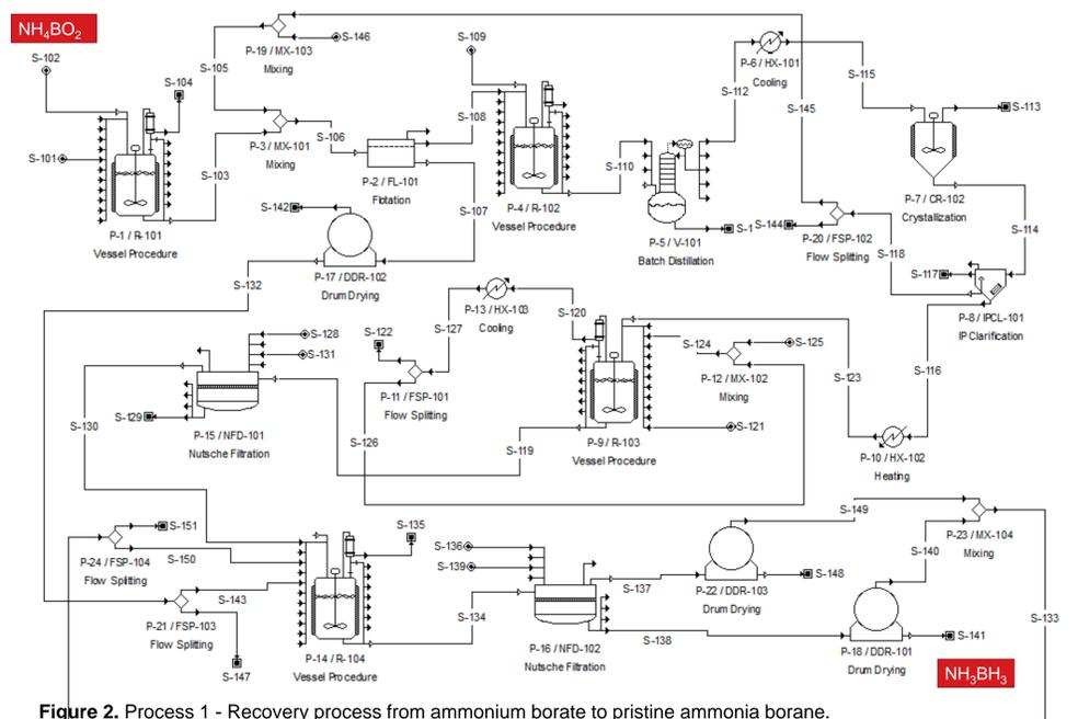
Figure 2. Process 1 - Recovery process from ammonium borate to pristine ammonia borane.
