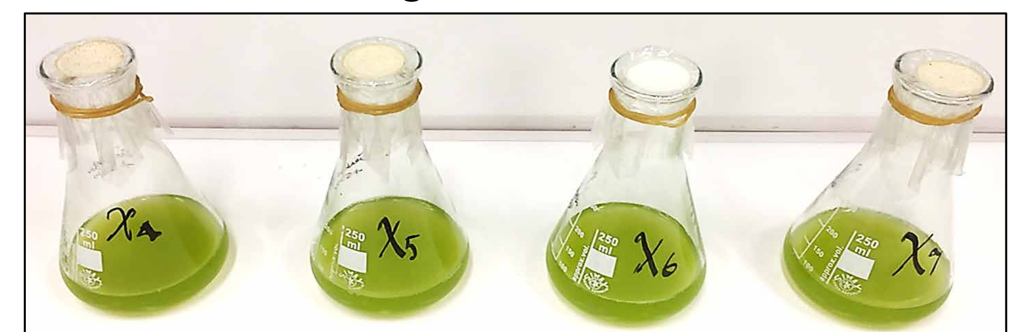
X4:0.5%; X5:2%; X6:10%; X7:0% organics in mixture of FO concentrated SDW + seawater at Day 25
